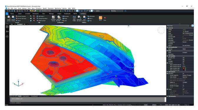
There are commands for interactive editing of the surface, and it also offers tools for detecting and repairing errors. Surfaces can have multiple boundaries or islands, and can be drawn as lines, 3D faces, or meshes.
