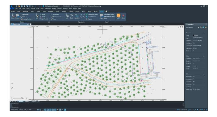
It is also possible to create new points from CAD entities drawn by other programs. If codes have been assigned to points in the field, the program will automatically draw the planimetry and blocks defined by the user. In addition, we can run all kinds of editing and filtering operations.
