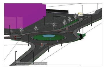
a best-fit alignment based on existing road centerline or road edge survey data. Superelevation calculation features a comprehensive definition and editing tool. Plateia supports several superelevations definitions and pivot point options according to various European and AASHTO roadway design standards. A number of alignment labels according to different country standards, reports, and data export options offer the flexibility to cover a wide range of user requirements.
