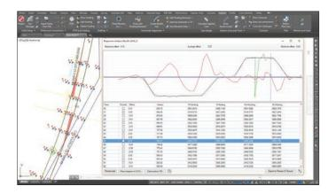
Options for converting surveyed rails to centerline review and edit regression points with point exclusion or inclusion in regression analysis lead to significant improvements in alignment or profile best-fit geometry. Multiple diagram options give users detailed information on curvature, transition areas, applied cant, and slew. All regression data is dynamically updated when changes occur.
