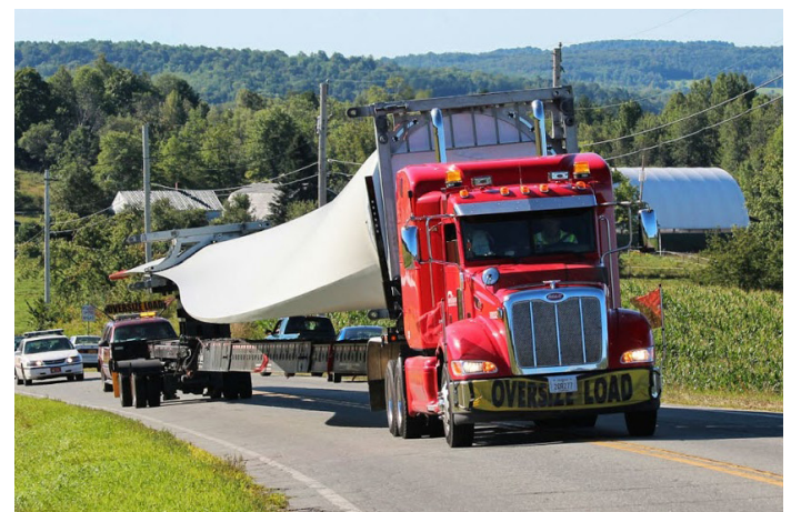
The turbines required for the Kingdom Community wind farm actually stopped traffic briefly on their way to their final destination. The trucks needed both lanes of a two-lane highway to allow for the wide turns at some of the intersections.
