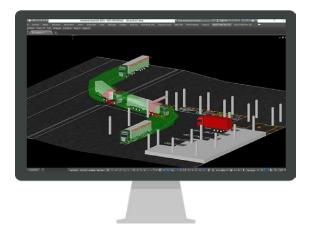
AutoTURN® is a swept path simulation and analysis software that helps you test vehicle movements in your road and site design projects. Whether you are involved in the design and planning of roundabouts, junctions, car parks, loading bays or bus terminals, AutoTURN® ensures that the planned layout can safely accommodate the expected vehicle manoeuvres and turning radii.
