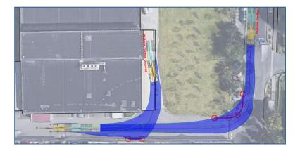
Real-time visual feedback when AutoTURN detects conflicts between a vehicle simulation and objects in the drawing.
